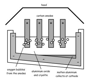
The sides and the bottom of a steel tank are lined with carbon. The carbon lining is connected to an electricity supply to make the cathode. The anodes are also made of carbon. They are lowered into the molten mixture of aluminium oxide and cryolite.
